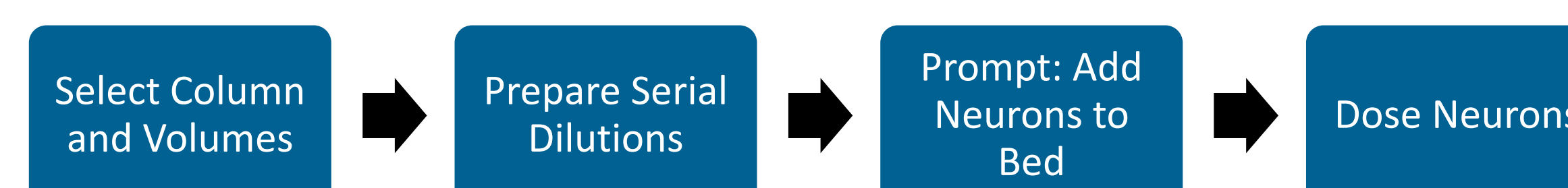
Figure 3. PIPETMAX Workflow for Serial Dilutions and Dosing Each run prepares an eight-point, 10-fold serial in the dilution plate of one user-defined column of the "Compounds" plate. Upon completion of the serial dilution the user is prompted to place the neurons on the bed. An option to run a second set of dilutions is available.
