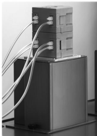
**GX Rinse Pump on the locator plate of the liquid handler**
