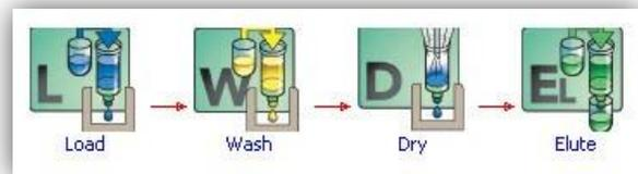
Figure 3. TRILUTION® LH THC Solid Phase Extraction Method Using the Gilson GX-274 ASPEC™ System
